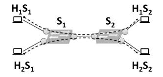
The case with separate queues experiences lower average per-packet delay due to lack of interference
