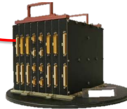
Remote Interface Unit
