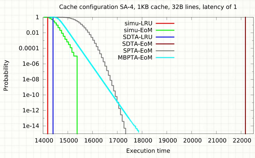
SPTA-EoM and MBPTA-EoM: strictly higher than simu-EoM & pWCET estimates between SDTA-LRU and SDTA-EoM<sup>26</sup>
