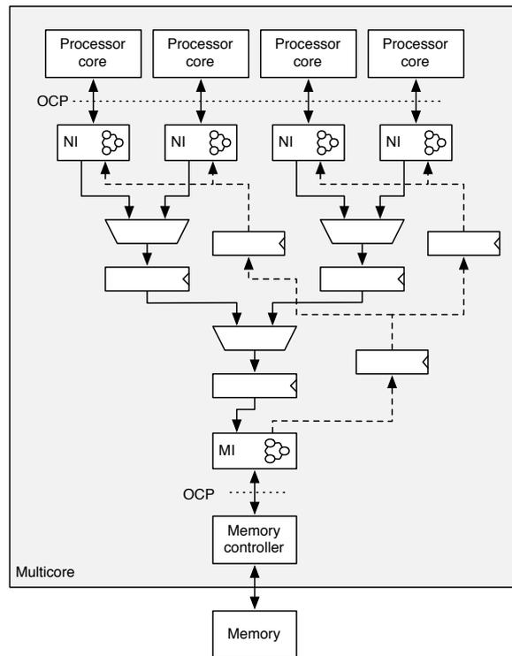
■ **Figure 2** The distributed TDM based memory NoC.
